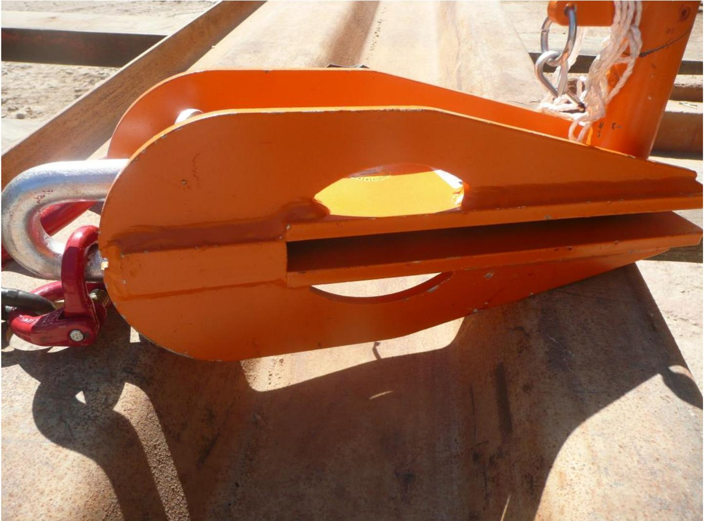
Mandatory accessory for jobs requiring handling of sheet piles or sheet piling, this clamp secures automatic dropping of sheet pile or pile away.
