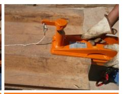
Drag the clip to the hole in the sheet pile.
