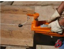
Unlock the bolt by a single 180° rotation.
